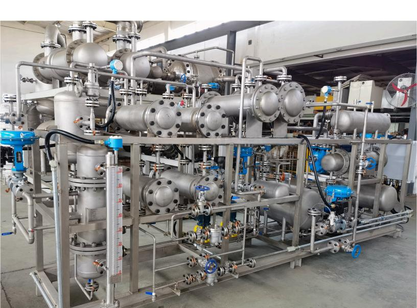
SOLVOSEP excels in applications where traditional separation methods struggle. By employing advanced pervaporation membranes, SOLVOSEP can tackle complex solvent mixtures and produce streams with varying impurity levels. This technology addresses challenges in separating azeotropic mixtures and enhances the overall efficiency of solvent recovery processes
